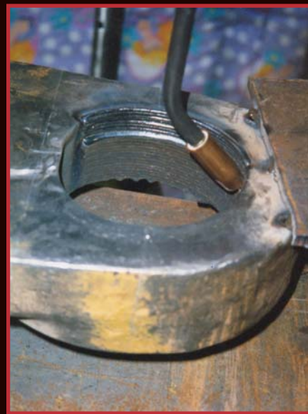
"Pie Mode" weld utilizing Bortech's Auto-Skip function.
