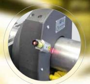
Integrated line laser to determine the cut off point.
